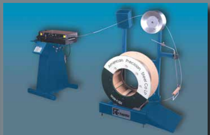
Complete cut-to-length line: SCL125S + CB16A + W6S air feed CTL machine and RD317S rim drive payout reel (loop is developed behind and above reel to save space).
